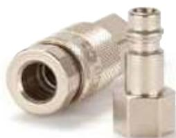
This coupling system has been developed specifically for the area of breathing protection. Coupling system with single-hand operation. High Flow valve for optimum flow and low pressure drop. Additional safety locking system. This safety lock prevents unintentional disconnection. To disconnect, the plug must first be pushed further into the coupling before it can be unlocked. Tested according to DIN EN 14593.
